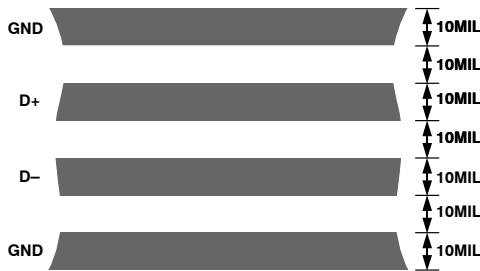
Figure 19. Arrangement of Signal Tracks
