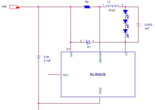
A value of 1uF will reduce the supply ripple current by a factor three (approx.). Proportionally lower ripple can be achieved with higher capacitor values. Note that the capacitor will not affect operating frequency or efficiency, but it will increase start-up delay and reduce the frequency of
