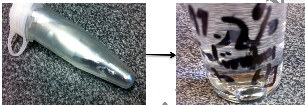
Figure 21. Left: Ga alloy sticking to eppendorf. Right: 11.2%wt galinstan: Hg, combined under deaerated 0.1\text{mol dm}^{-3} KCl
