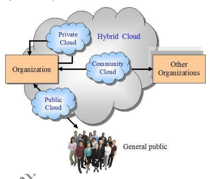
Figure 7 Cloud computing deployment models.
