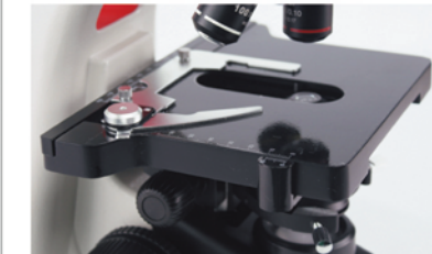
Double-layer mechanical stage, with double slide clips
